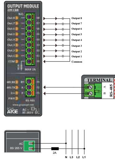
RT Terminal Block: It is used for optional activation of 120  $\Omega$  terminating resistor.
