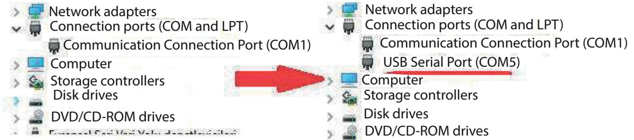
2. The port opened by the connected RS-485 converter on the computer is selected with the "New" button at the top left.
