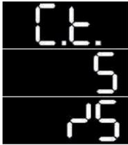
After giving energy to the device, the current transformer ratio menu in Figure 2.1 will appear. In this screen, the current transformer ratio is set with the direction buttons and is confirmed with PRG button.
