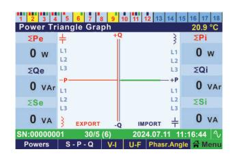
The blue-dashed section represents the inductive and capacitive values for the import power triangle. Each of the four quadrants displays the status of the phases (L1, L2, L3), indicating which phase is active in that specific quadrant.
