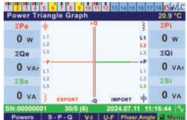
The blue-dashed section represents the inductive and capacitive values for the import power triangle. Each of the four quadrants displays the status of the phases (L1, L2, L3), indicating which phase is active in that specific quadrant.
