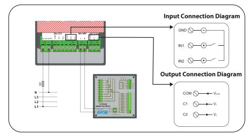
**GSM AUTOMATION TERMINAL - METER (RS-485) CONNECTION DIAGRAM**
