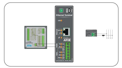
**EHTERNET TERMINAL - METER (RS-485) CONNECTION DIAGRAM**
