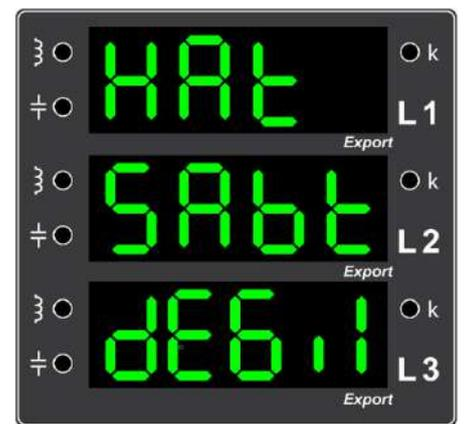
**Example Error 24.** Screenshot indicating that the stage has exceeded the pull-up/release limit
