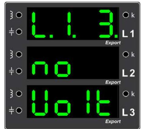
**Example Error 6.** Screenshot showing that the voltage inputs of the first and third phases are empty
