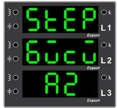
**Example Error 18.** Screenshot indicating that the installation could not be completed with the available stages
