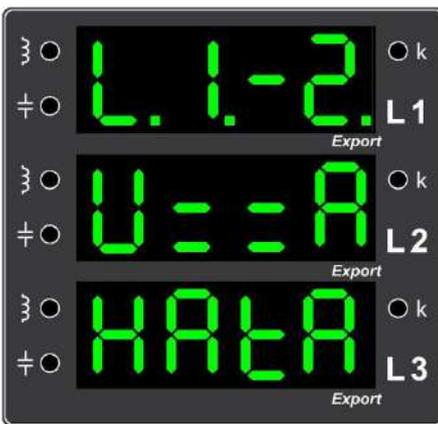
**Example Error 22.** Screen display showing that the voltage-current terminals of the 1st and 2nd phases are not matched when automatic voltage-current matching is off
