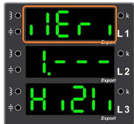
Figure 2.3. "Advanced" access level seen on the first line when entering the menu
