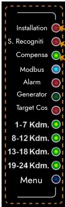
Figure 6. From the Status LEDs on the left side of the device, the "K.Recognition" LED is set to lights up continuously during recognition.
