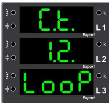
**Example Error 16.** Screenshot showing that the current transformer terminals of the first and second phases are connected by mixing them to form a loop
