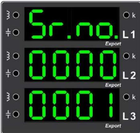
**Figure 1.** The first opening screen showing the "Serial Number" of the device
