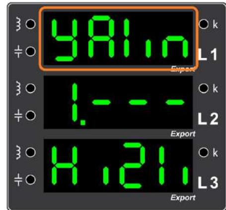
Figure 2.1. "Lean" access level seen in the first line when entering the menu
