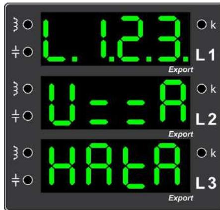
**Example Error 23.** When automatic current-voltage matching is off; screenshot showing that the voltage-current terminals of all phases are not matched
