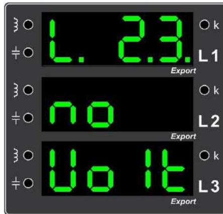
**Example Error 5.** Screenshot showing that the voltage inputs of the second and third phases are empty
