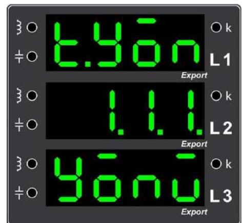
**Figure 4.** Screenshot of "Current Transformer Secondary Directions" detected by the device during installation
