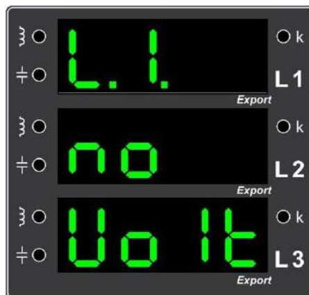
Example Error 4. The screenshot showing that the voltage input of the first phase is empty (Check the voltage connection of the first phase.)
