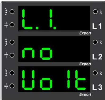
**Example Error 4.** Screenshot showing that the voltage input of the first phase is empty
