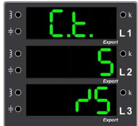
**Figure 2.** Screen display that shows the current transformer value (Current Transformer Value) in X/5 format
