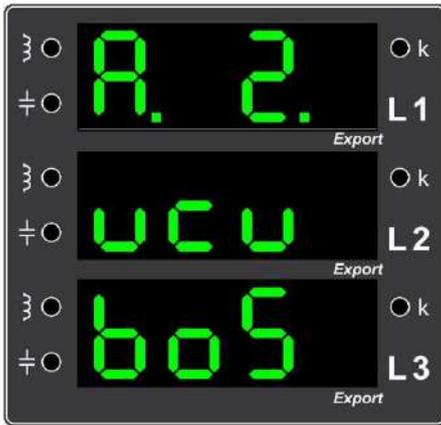
**Example Error 10.** Screen display showing that the current input of the second phase is empty
