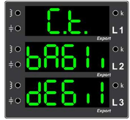
**Example Error 15.** Screen display showing that the current transformer is not connected
