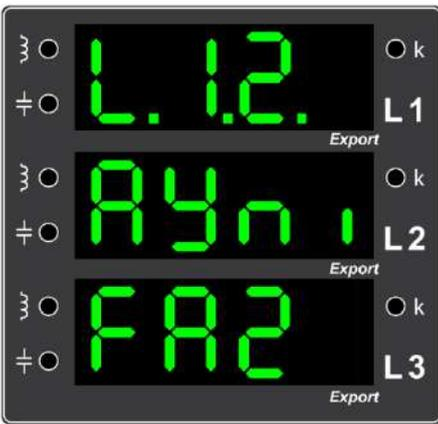
**Example Error 19.** Screenshot showing that the voltages connected for the first and second phases are in the same phase
