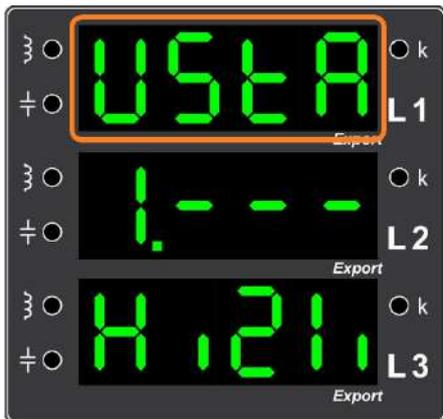
Figure 2.2. "Master" access level seen on the first line when entering the menu
