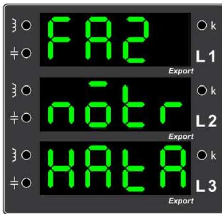
**Example additional Error 13.** Screen display showing Phase/Neutral connection error
