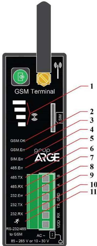
1. **4 level LED:** It indicates GSM signal quality. If all 4 are on, it has the best signal. If a single LED or none is on, it is recommended to amplify the signal with a wired antenna (ANT 03 or ANT 07).
